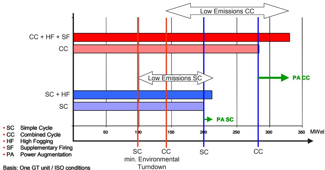
Figure 5.3: SC13E2 / KA13E2 high power output flexibility
