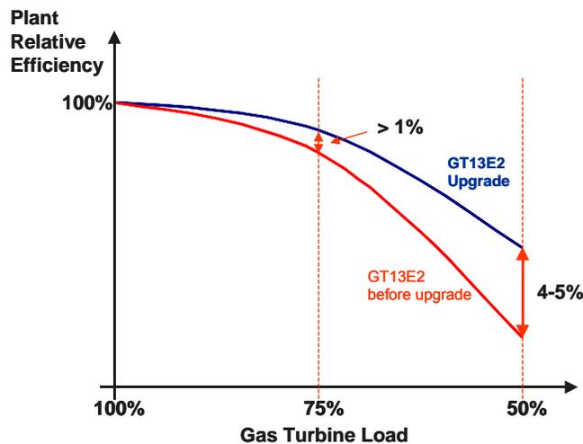
Figure 5.1: KA13E2-2 part load behaviour
