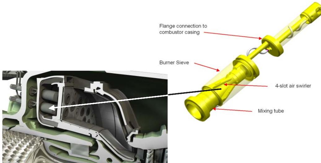
Figure 4.3: AEV burner design features
